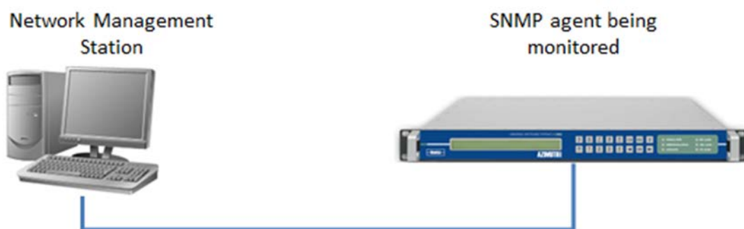
Figure 1 - SNMP Management System
