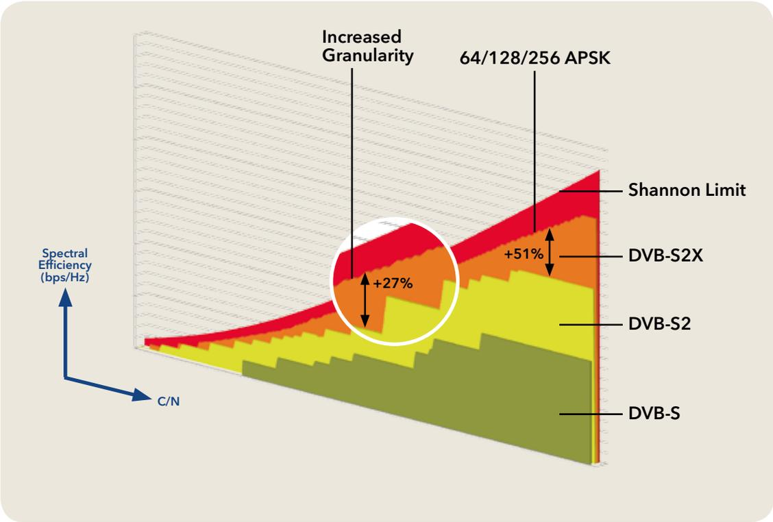
DVB-S2X compared to DVB-S2 (64/128/256APSK & increased granularity)
