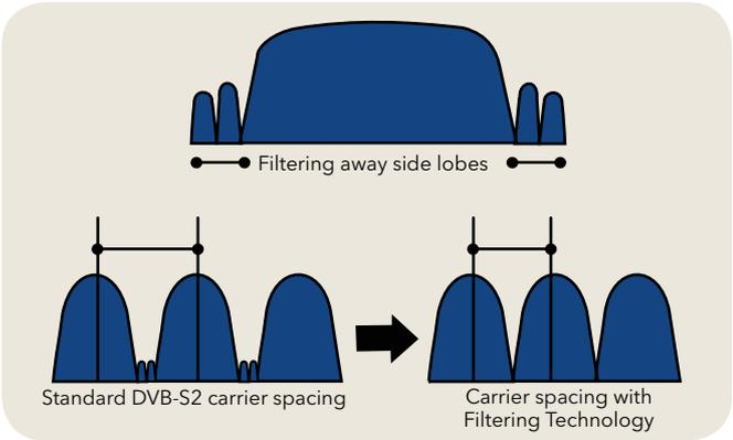
**Optimal Carrier Spacing**
